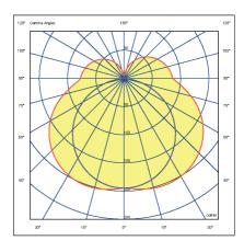
R LUM W: Installation for a clean room with distribution light lambert and low UGR index.
